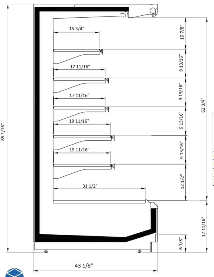
High Volume Bulk Convertible Merchandiser with Six Display Levels, Extended Canopy and Low Front
